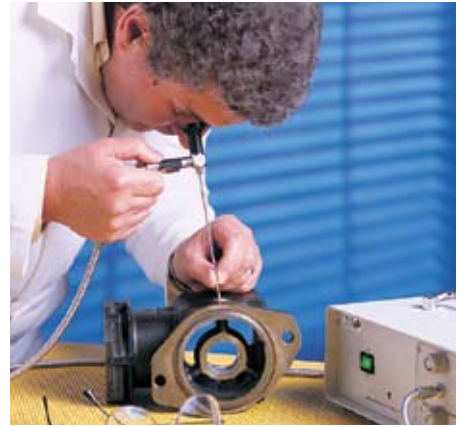
Inspecting air-brake compressor after machining
