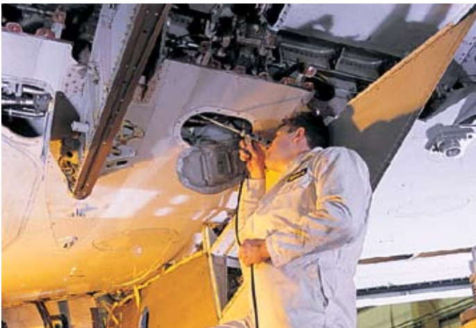
Inspection of hard-to-reach area of airframe structure
