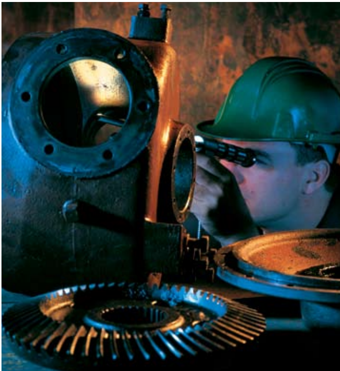
Rigid Borescope inspection of power take-off transmission
