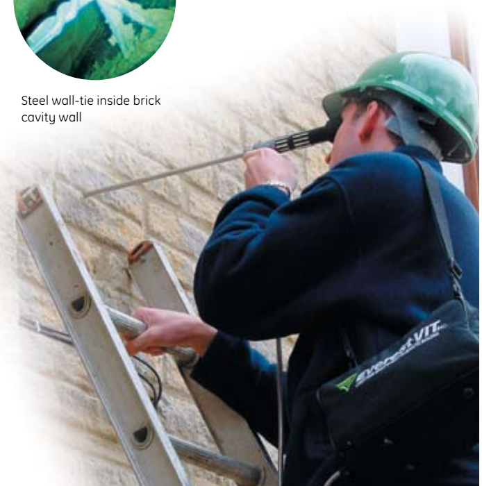
Structural surveying with fully portable ELS-24DC KIT, light source and battery pack.
